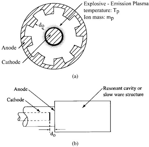
Fig. 1. The model proposed is applicable to both (a) cross-field microwave devices such as the magnetron and MILO, as well as (b) linear beam sources such as the virtual cathode and the backward wave oscillator.
