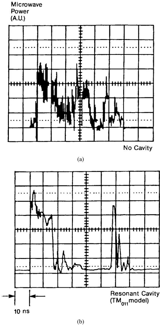
Fig. 7. Data (from [19]) showing the (a) overmoded and (b) resonant cavity vircator output pulses. The cavity vircator microwave pulse width decreases (relative to the free-running, overmoded configuration) as the virtual cathode frequency chirps to a region of frequency space that the cavity boundary conditions cannot support.
