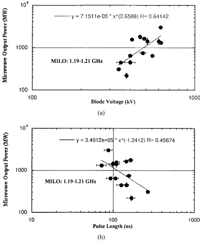
Fig. 5. (a) Microwave power versus diode voltage and (b) microwave power versus microwave pulse length scalings for an *L*-Band magnetically-insulated line oscillator.
