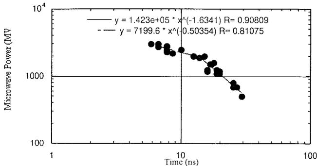
Fig. 6. Microwave power versus microwave pulse length scaling for an *X*-Band backward wave oscillator.
