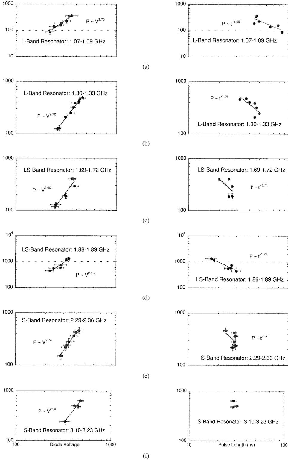
Fig. 4. Microwave power (MW) versus diode voltage (kV), and microwave power versus microwave pulse length (ns) scalings for a suite of four tunable relativistic magnetrons. Power law fits to the data are summarized in Table I.
