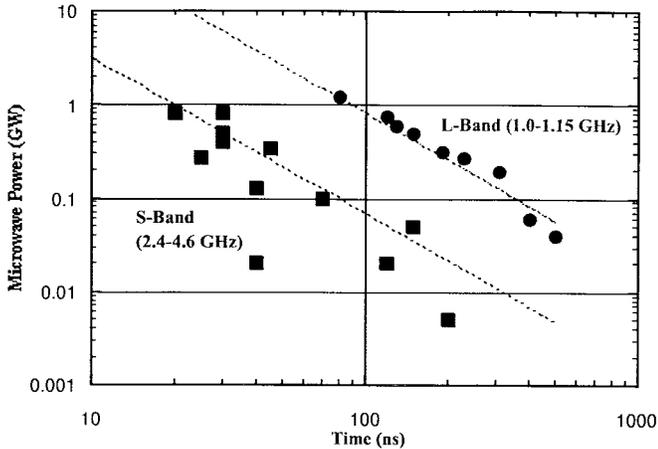
Fig. 3. Both *S*-Band and *L*-Band magnetron data from a number of different laboratories (MPI, MIT, NCSU, SRINP, NRL, Stanford Univ., Rafael, Varian and T-CSF) exhibit a power versus pulse length scaling consistent with the model (the curves are fits to  $P \propto \tau^{-5/3}$ ) based on cathode plasma motion proposed herein.
