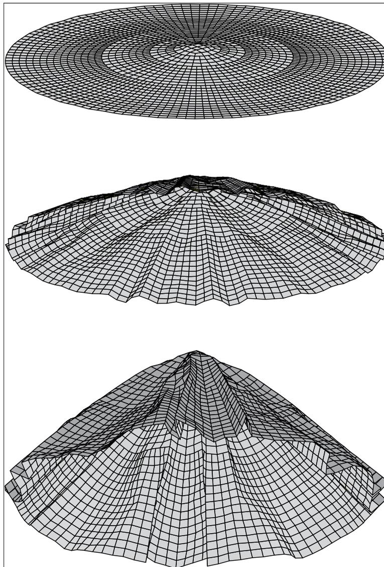
**FIGURE 2. Deployment Of A 1 Meter Sail By Centrifugal Force.** We are carrying out deployment demonstrations and simulations by several different physical mechanisms. Sail has stiffness and mass density of the carbon micro-truss sail material, and microwave pressure supports it against gravity. Simulation snapshots show large-deformation and folding is corrected by spins of 0.5, 1.0, and 2.0 revolutions/sec (bottom to top). Spin is necessary for rigidity of sails without structural stiffening.
