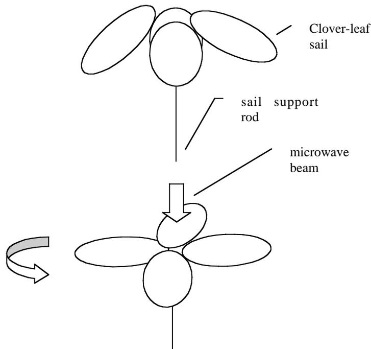
**FIGURE 1. Schematic Of Experiment Demonstrating Spin Deployment: Opening Of Cloverleaf Sail By Electrodynamic Spin-Up.** Above, the sail droops before beam it turned on. Below, with the beam on, the sail spins, deploys: The clover-leaves open upward against gravity, supported by centrifugal acceleration.
