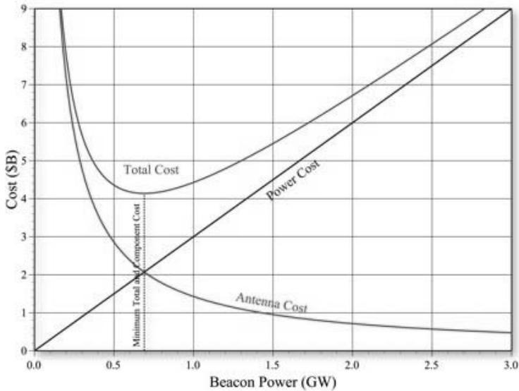
**Fig. 1.** Antenna, microwave power and total costs of Beacon with effective isotropic radiated power of 1017 watts. Cost is in billions of dollars, and power in gigawatts (109 watts, the power of a large nuclear reactor). It radiates at frequency 1 GHz and has costs typical of ours today. Minimum total occurs when the antenna cost and power cost are equal.
